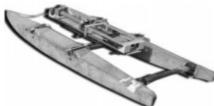
new type of device promising to extract energy from wave power. The concept uses a floating catamaran optimised to be laterally stable but rock longitudinally. A mass is free to move up and down the length of the deck, acting as a piston as it reaches each end of its travel. Fluid displaced by the piston generates power. Alternatively, the piston could be replaced by a
