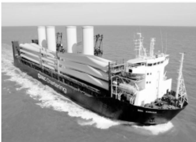
Each bottom tower section, which is on deck in an upright position, weighs 90 tonnes and is 25 m high. The forward position of the BBC Konan's bridge means that the upright towers do not obstruct the crew's view. The wind turbine blades measure 52 m in length, and the nacelles with the pre-mounted hubs are the heaviest pieces, weighing 177 tonnes each.
