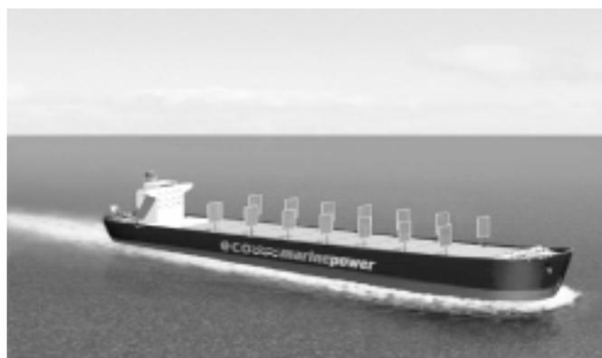
the energy provided by wind and sun. The array of rigid sails are also solar panels, always kept in optimum position by a computer control system developed by KEI System Pty Ltd of Osaka, Japan, whereby intervention by the crew is kept to a minimum. When wind conditions are not favourable the solar sails can also be positioned to offer little wind resistance and yet still collect solar energy. The sails may be used when the ship is at anchor or in harbour or can be lowered and
