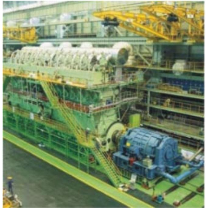
Available in 6-cylinder up to 14-cylinder configuration, the Wärtsilä RT-flex96C and RTA96C low-speed engines cover a power range from 24,000 to 80,080 kW at 92 to 102 rpm.
