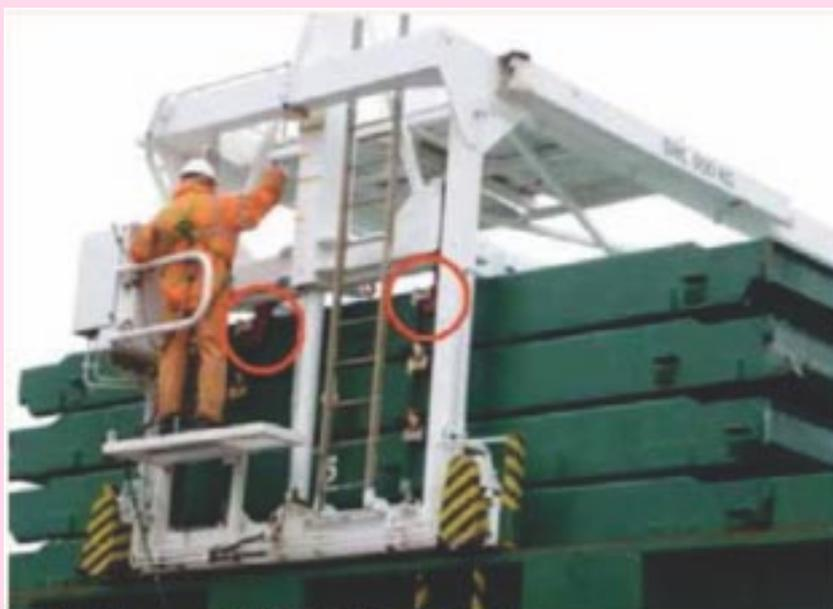
The hatch crane with hatch in hooked position
