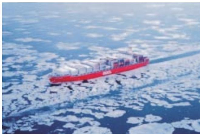
by chunks of ice which may be 50 centimeters or more in thickness. Not only is the ice highly abrasive, there is the additional factor that the steel of the hull flexes under the impact.
