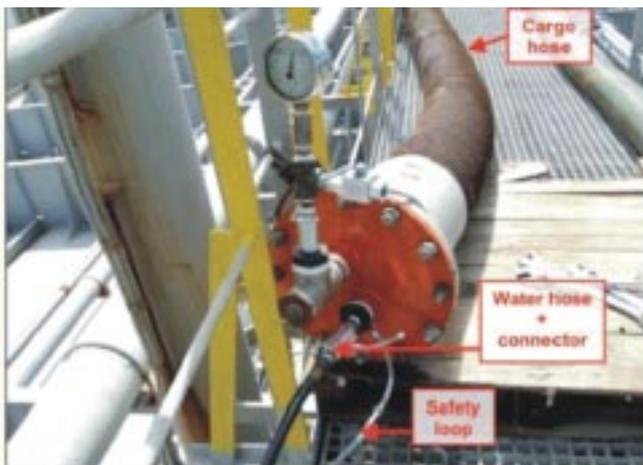
▲ Safe cargo hose pressure-testing arrangement showing safety loop across connector between water and cargo hoses
