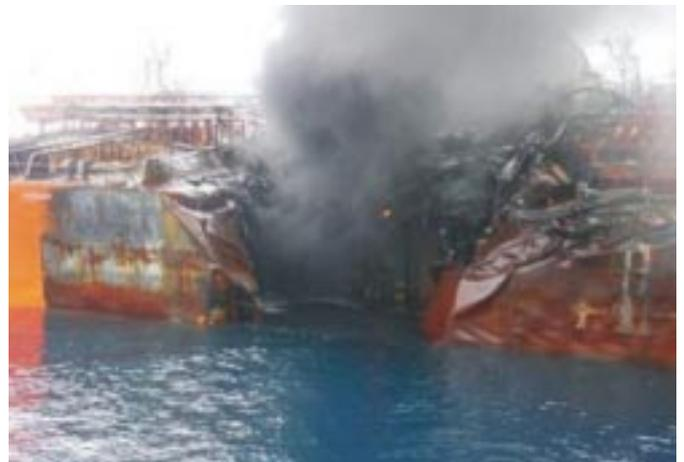
combination of the collision damage and fire has severely weakened the local and global structural strength of the ship. The prolonged exposure to swells of up to four metres may also have contributed further damage and continued exposure will only make this worse.
