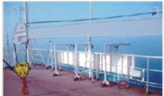
Slewing the crane over the compass deck permits safer access to the jib
