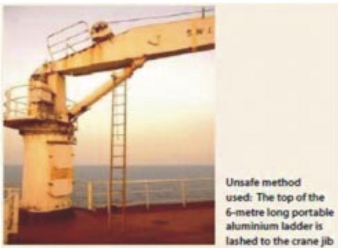
Unsafe method used: The top of the 6-metre long portable aluminium ladder is lashed to the crane jib
