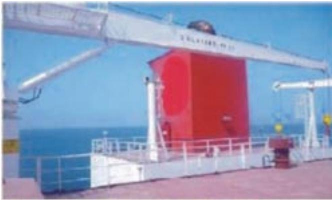
Post-maintenance photo showing the crane raised from stowage crutch and slewed over the bridge deck, permitting safe and efficient access from portable scaffolding
