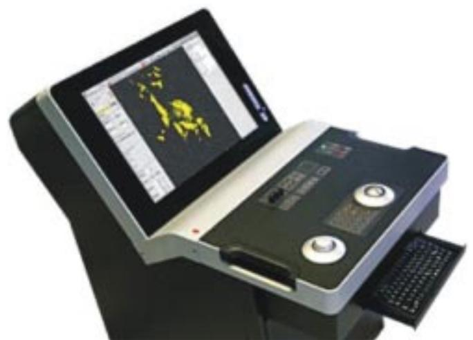
**6. Automatic Tracking Aid:** Just like ARPA, automatic tracking aid displays the information on tracked targets in graphic and numeric to generate a planned layout for a safer and collision free course.
