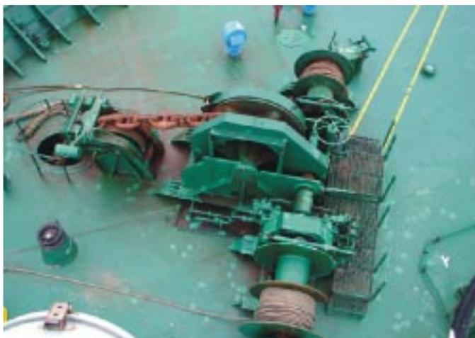
**5. Check Brake Linkages:** The brake linkages should be checked for free movement. If the linkages are not free then there would be a loss of brake holding capacity. This would create a wrong impression to the operator that the brake has been applied fully, but in fact has not or the brake mechanism is hardened up from lever bars, which have a tendency to build up high stresses on some mechanical parts of the brakes.
