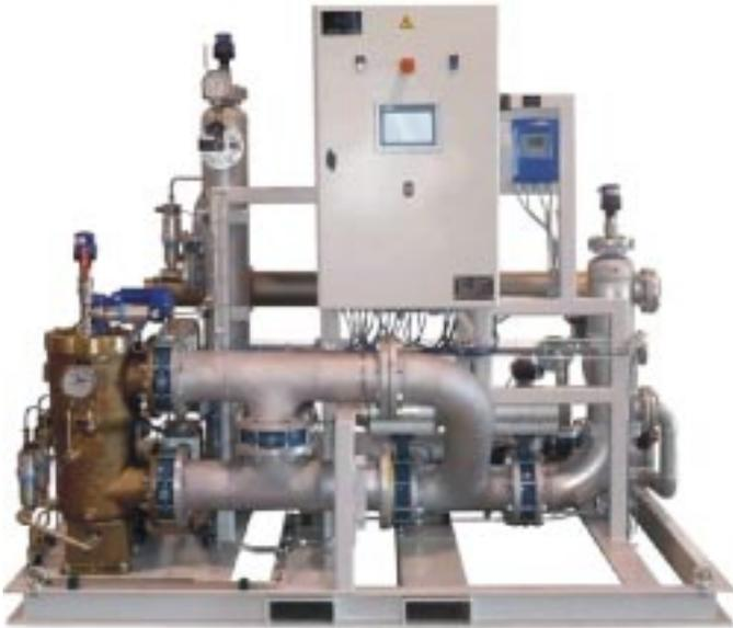
means of UV-C light. 'This happens at 254 nanometers, the optimal wavelength for UV-C light to render micro-organisms inactive. The light penetrates the core of the DNA, and subverts the metabolism of the cells', explains Xavier Deval (Business director Bio-Sea). He continues: 'What is most important is that the correct UV dose is applied. Otherwise the ship will not comply with regulations, because the water is not correctly treated.'
