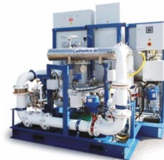
hr per lamp) and is designed to make the sea water flow along one side and then the other - doubling UV exposure. In addition, the manifolds make the water flow in a helix, ensuring that the maximum surface area is exposed to the UV light source.
