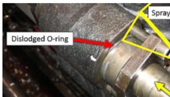
On November 25, 2015, the Gunde Maersk's three auxiliary generators began to leak fuel when switching over to ultra-low-sulfur diesel.
