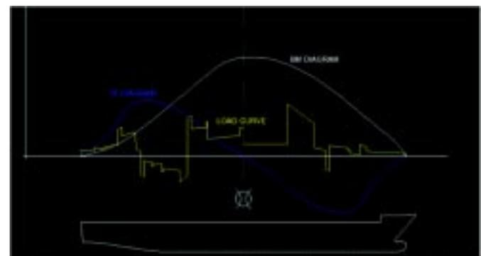
Figure 3: SF and BM Diagrams of a ship
