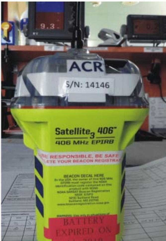
Confirm the expiry dates of pyrotechnics, LTA, HRU, EPIRB, GMDSS batteries, MOB marker, Lifejackets and immersion suit lights
