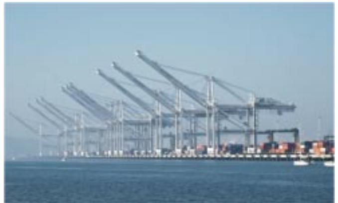
The cranes are used to load and unload container vessels. The Port said taller cranes will be better able to reach containers stacked high above decks on modern-day megaships.
