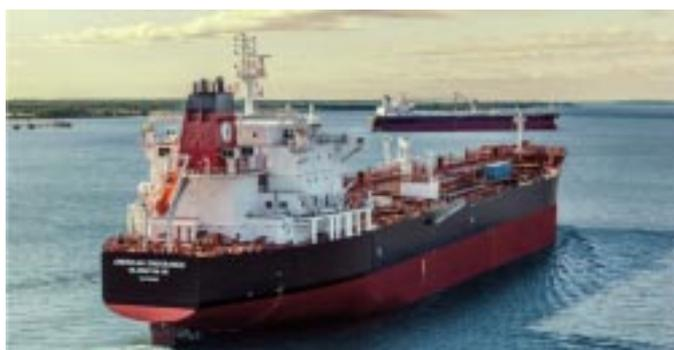
The next generation 50,000 dwt product tanker is based on a proven Hyundai Mipo Dockyards (HMD) design that also incorporates numerous fuel efficiency features, flexible cargo capability, and the latest regulatory requirements. The vessel has also received LNG Ready Level 1 approval from the American Bureau of Shipping (ABS). The 600-foot tanker has a carrying capacity of 14.5 million gallons of crude oil or refined products.
