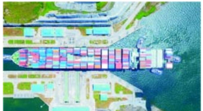
The vessel measures 351 meters in length (long) and 43 meters in length (width) with a carrying capacity of 9,504 TEUs (20 foot containers).
