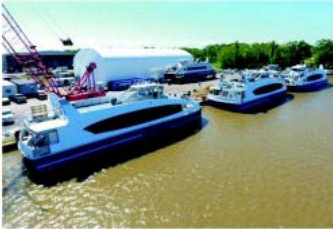
NYC Ferry's new USCG Subchapter K vessels are designed by Incat Crowther and powered by twin twelve-cylinder, 1,400-horsepower Baudouin 12M26.3 diesel engines, coupled to ZF Marine ZF3050 gearboxes and turning custom five-blade Michigan Wheel propellers. These larger "Rockaway Class" vessels boast an operating speed of 24 knots.
