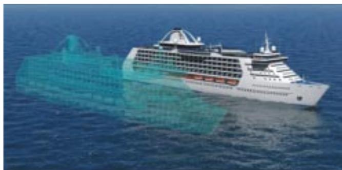
A digital twin is a digital copy of a real ship, including its systems, which synthesizes the information available about the ship in a digital world. Using digital twins enable optimization of a ship's design, maintenance, production and sustainability throughout its entire lifecycle.
